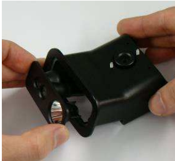
Figure 6: Step 3 - push the front panel with optic into the housing
